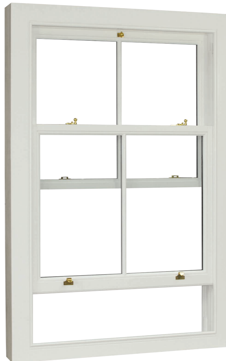
Window as shown: One over one traditional box sash window with brass fittings and standard bead and astragal bar. Paint finish is white to interior and exterior.
