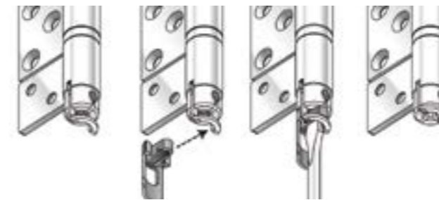
Figure 38: Vertical adjustment with shipping clip
